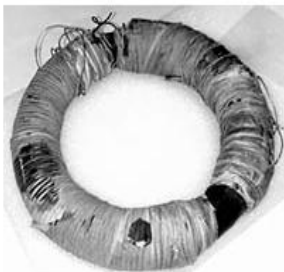
Photo of one of Michael Faraday's original wire-coiled iron rings, courtesy of the Royal Institution, where Faraday did his experiments
