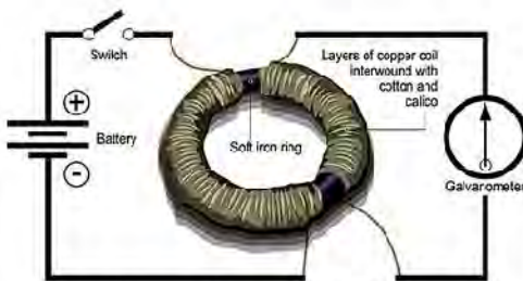
Diagram showing the basic set-up of Faraday experiment.
