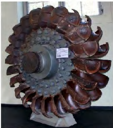
Old Pelton wheel from Walchensee Power Plant, Germany
