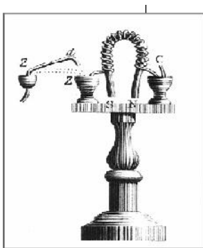
The first artificial electromagnet, invented by Sturgeon in 1824. Sturgeon's original drawing from his 1824 report to the British Royal Society of Arts, Manufactures, and Commerce. The magnet was made of 78 turns of bare copper wire (insulated wires had not yet been invented).
