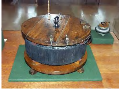
Prototypes of the world's first high-efficiency transformers. They were built by the Z.B.D. team on 16th September 1884.
