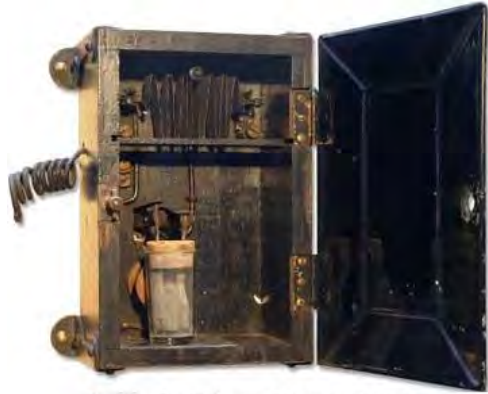
Inside the Edison Chemical Meter. Note the small jar containing the electrodes and electrolyte solution.
