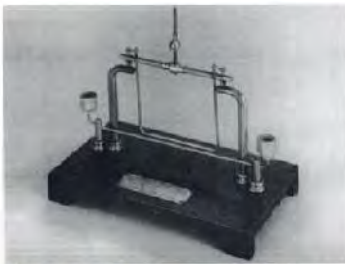
A reproduction of Ampere's apparatus for studying the interaction between two current-carrying parallel conductors.
