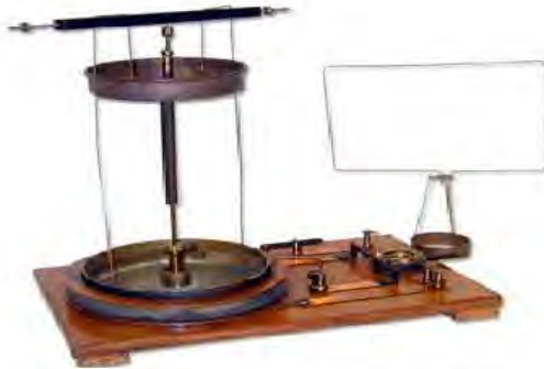
This is an early model of the same apparatus constructed by Ampere for his famous experiments on the relationship between magnetic fields and electric current.
