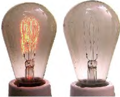
Carbon filament lamp (E27 socket, 220 volts, approx. 30 watts, left side: running with 100 volts)
